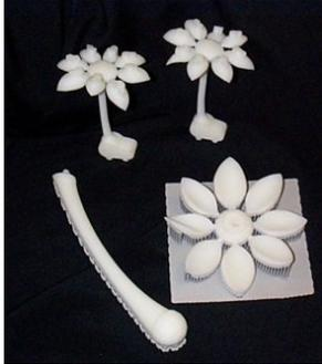
Figure 113: CALM project - final object produced by fused deposition modelling (Katie Bunnell). Reproduced by kind permission of the Learning Development Unit
