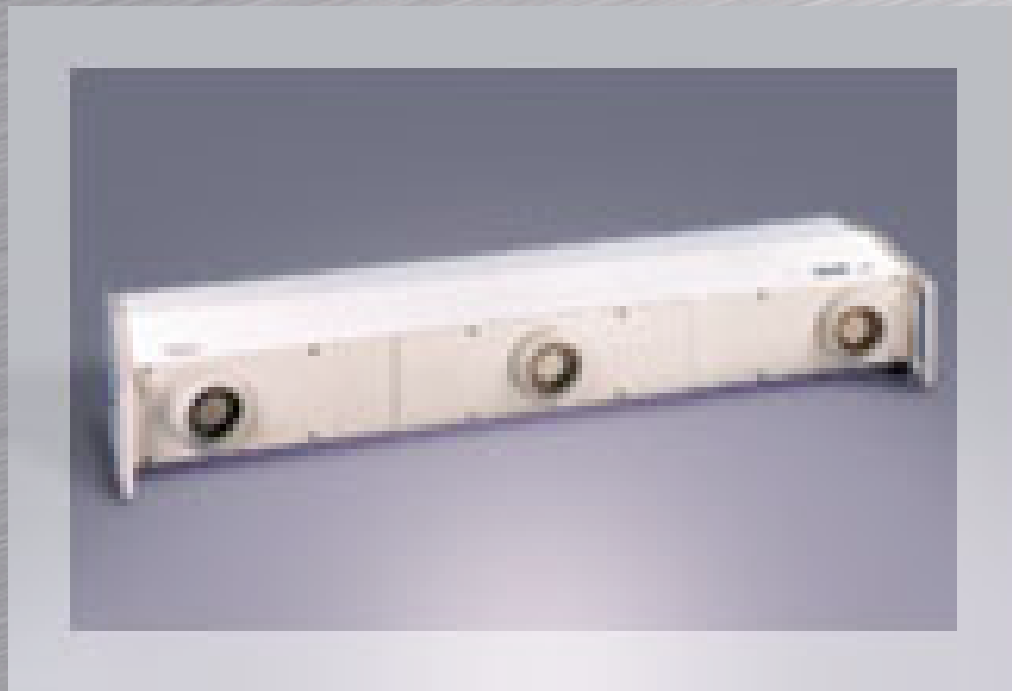
Optotrak - active marker system
