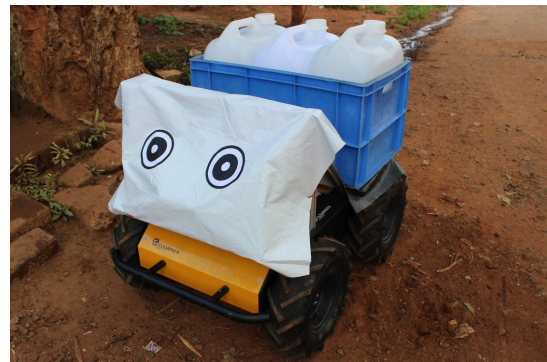
Fig. 2. Husky UGV robot fitted with a crate, loaded with cans
